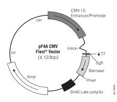
Figure 1. pF4A CMV Flexi® Vector circle map and sequence reference points.
