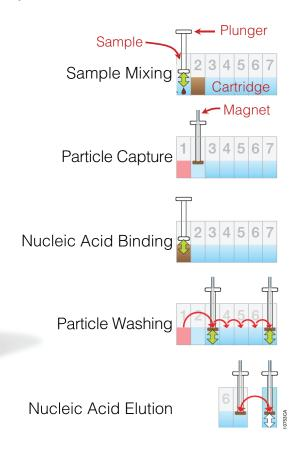
Magnetic particles are moved through the Maxwell cartridge wells.
