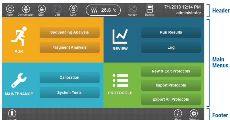
Figure 9. Spectrum Compact CE System Software Main Menu screen. The Header and Footer are fixed and remain available to the user across all menu screens. The navigation and informational icons displayed in these areas will vary depending on the specific workflow menu as well as selected security level.
